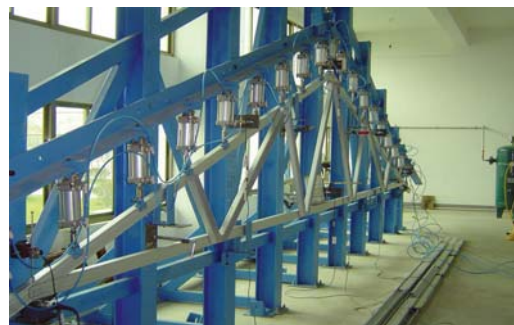
Top chord load test
